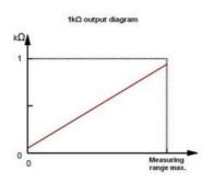
To ensure a good linearity, wire the potentiometer as a voltage divider and never as a rheostat. The input resistance of the operating system must be very high (greater than 10M $\Omega$ )
